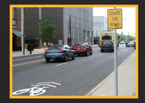
A shared lane marking, also called a sharrow, reminds motorists that bicyclists are sharing the traffic lane. It also guides bicyclists on where they should ride within the lane. Typically it consists of an arrow symbol, pointing in the direction of traffic, combined with the bike symbol.
