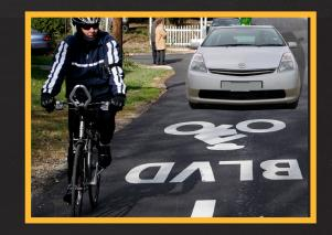
A bicycle boulevard is a low-volume, low-speed street, optimized for bicycle travel using traffic calming and traffic reduction treatments, signs and pavement markings, and intersection crossing treatments. Parts of streets, or a series of contiguous street segments, also can be a bike boulevard.
