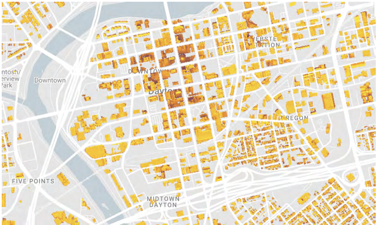
Figure 7. Rooftop solar potential in Dayton, where darker colors indicate greater levels of shading. Source: Sunroof Project. 23
