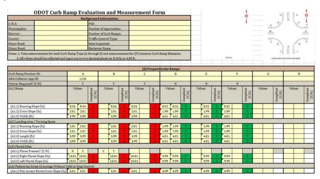
After filling in all measurements for curb ramp, if there is an "N" in any Compliant Column, then the ramp is noncompliant.
