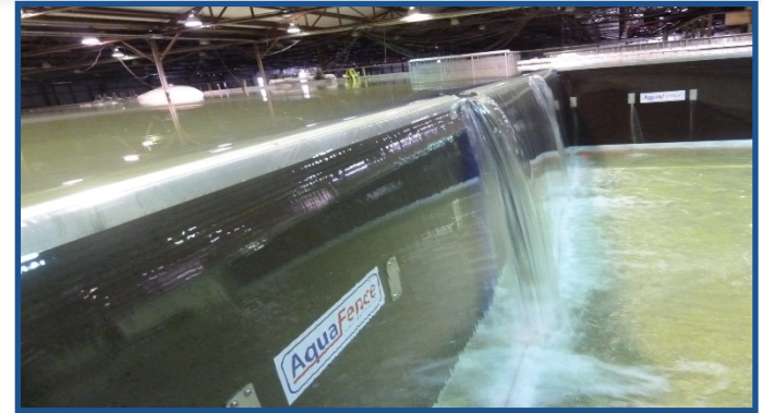
Overtopping test at ERDC. Water is brought to 1 inch above the barrier and allowed to overflow.
