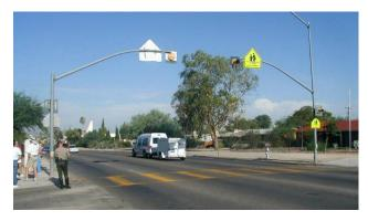
LED displays. These hang from a mast arm extending over the street. Some applications use flashing red or yellow beacons to enhance overhead signs, while at others, it is the pedestrian crossing sign itself that flashes. They can utilize passive or active actuation. Drawbacks of overhead flashing lights include higher-cost and the fact that they may not be immediately understood by motorists.
